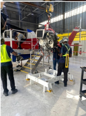
Cross Section of Caverton Engineers carrying out overhauling on the Twin otter engine at the MRO facility
